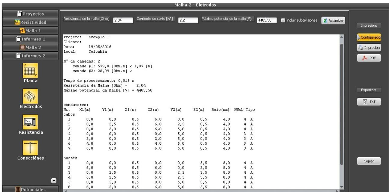
Note that the GPR (maximum grid potential) is obtained with the resistance and fault current values - if the current value isn't shown (or is the default of 1 kA), you have not entered it yet - go back to the admissible potentials screen, enter the value, then get to the electrodes table and click again on Calculate.
