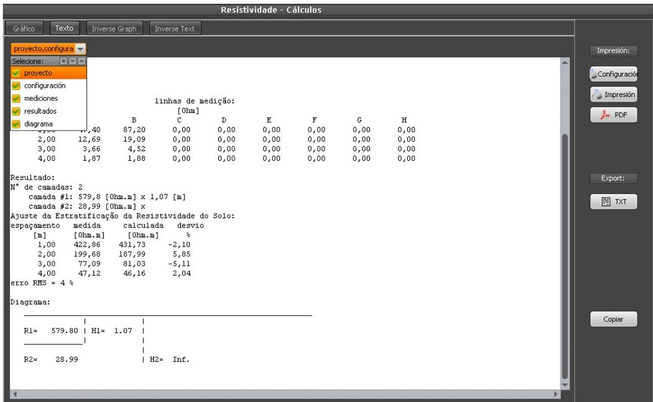
The stratification is considered satisfactory when none of the measurements have deviation greater than 15-20% and the full set of measurements has a RMS error below 10-15%.
