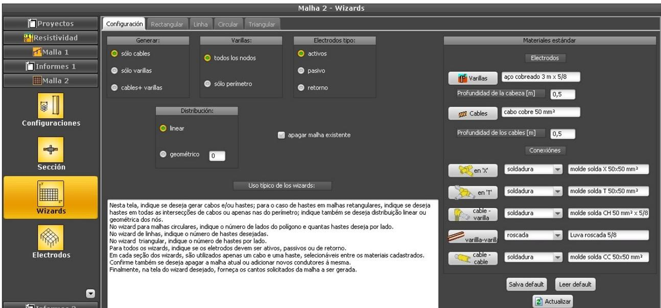
For this example, let’s generate cables + rods, with rods only at the border (perimeter) cable, active electrodes (see our tutorial on metallic fence for use of passive electrodes) and regular meshes (geometric division is used only in bigger grids).
