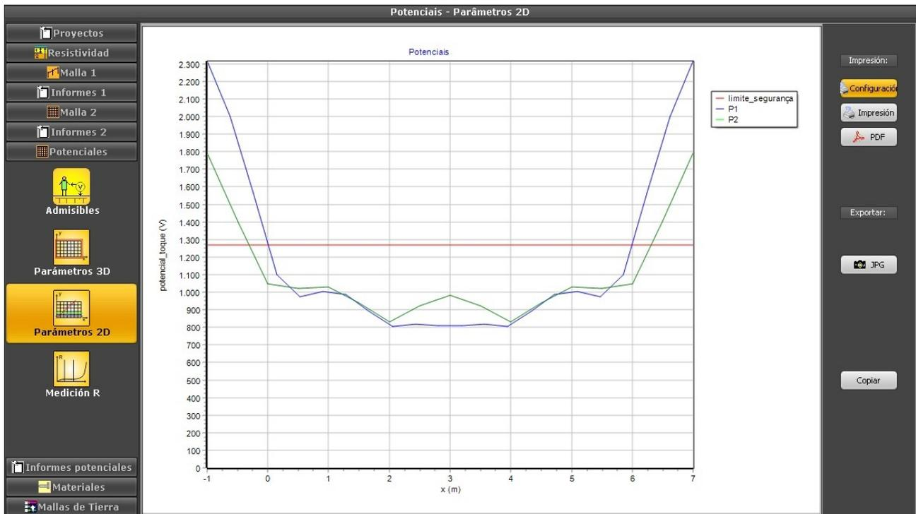
As can be seen, if the grid is for a closed brick structure with no metallic door, this grid is safe. If it's for an open substation with metallic fence, or a closed one with grounded metallic door, someone who touches these exposed parts from the outside would be in danger, even with the gravel layer. Let's see next what can be done to fix this.
