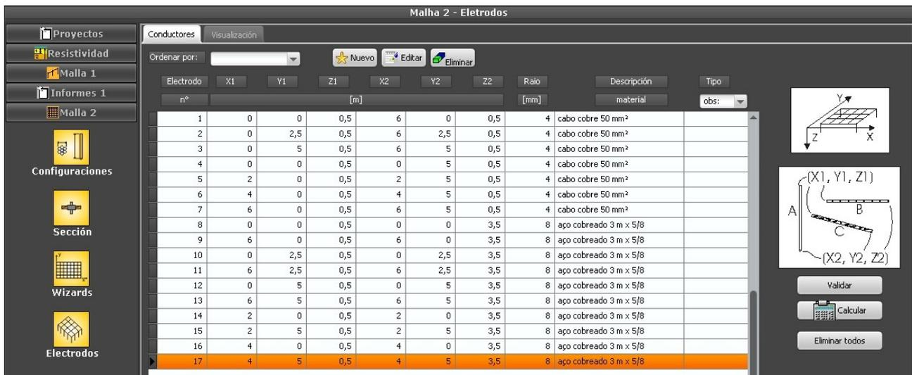
Note that, also here, the button Calculate isn't visible until you click at Validate - do that, then click on Calculate to get the grid resistance.
