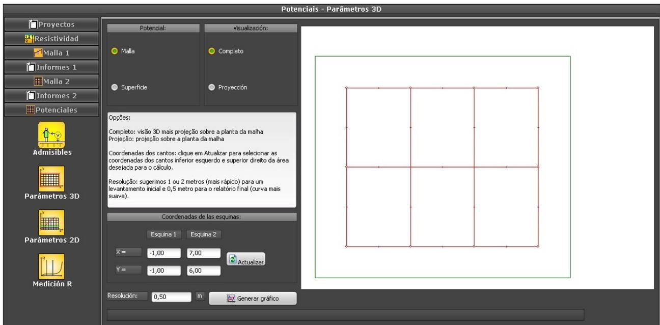
3D view of grid potentials - also available the surface potentials and, for both, the projection view:
