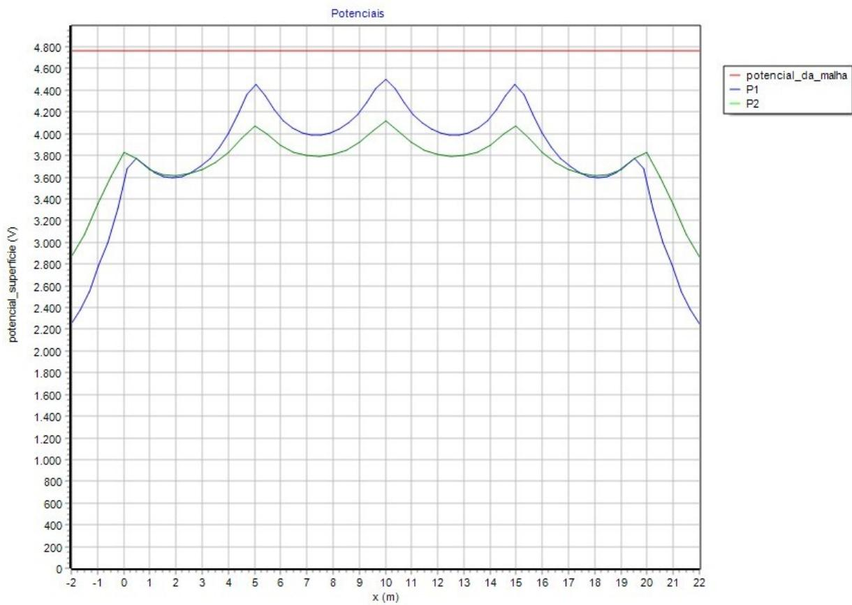
On the longitudinal direction (green line) we have the value of 2900 V at surface for X = -2 (foot potential) and 3277,8 V on the hand (potential elevation on passive electrode), resulting on a touch potential of 377,8 V.
