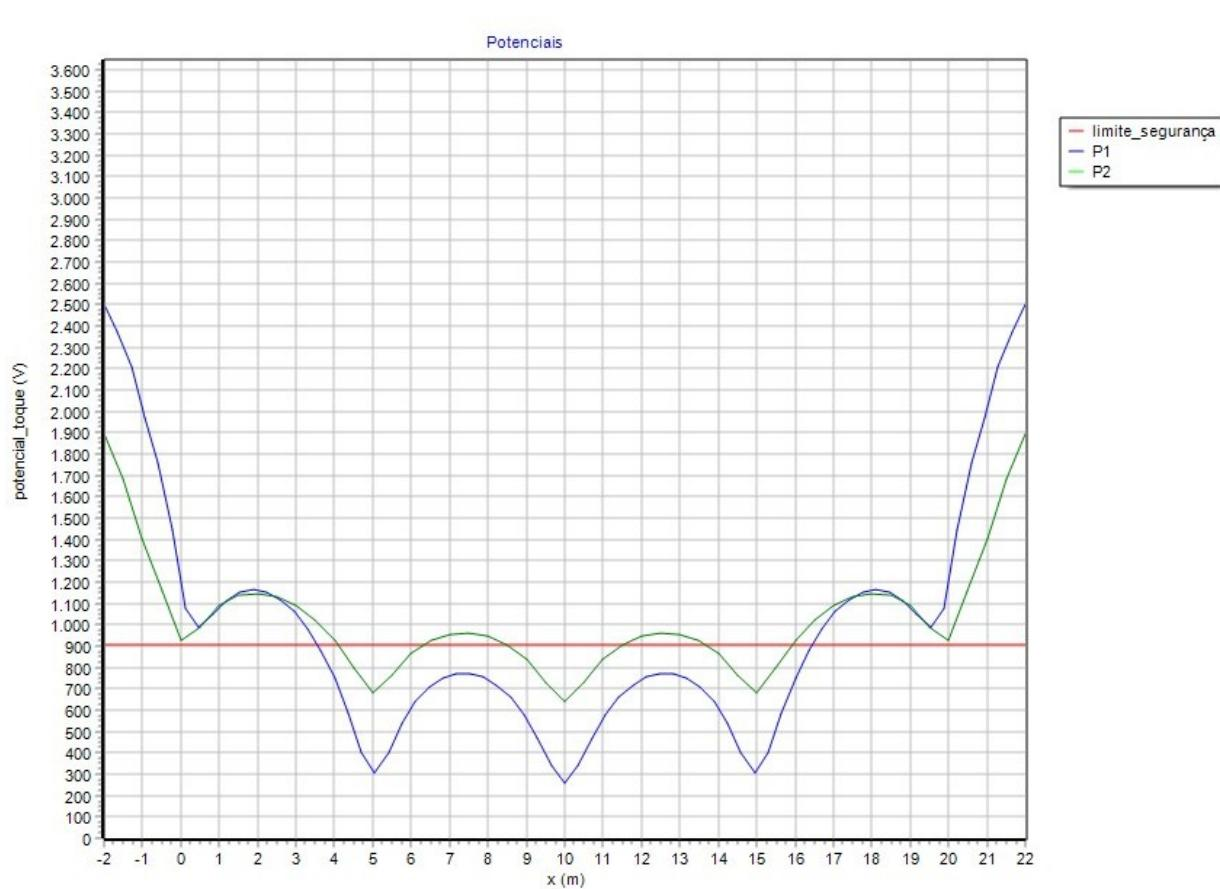
Again, the presence of the passive electrode doesn't affect the grid performance.
