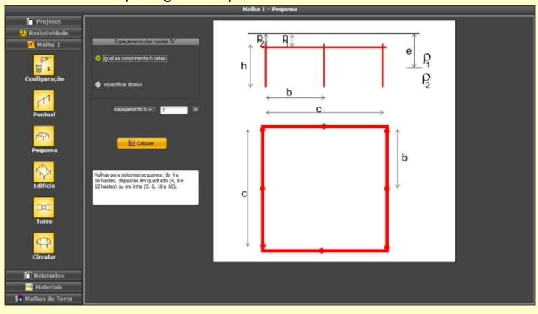
Besides the complex grid calculations in up to 4-layer soil on module Grid 2, the module Grid 1 gives you quick comparatives in 2-layer soil for several predefined configurations, like rectangular or circular (poligon) rings with up to 16 rods, with 3 rod lenghts
