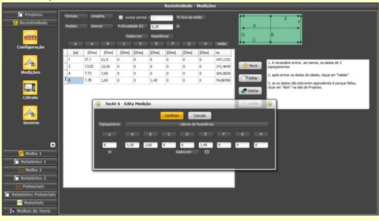
Using up to 8 measurement axis at a time, TecAt stratifies the soil in 2-, 3- or 4-layer model, with a numerical calculation, without the errors of graphical/manual methods - it not only gives you the best possible result, you can even check the errors of some stratification you got with another method or software!
