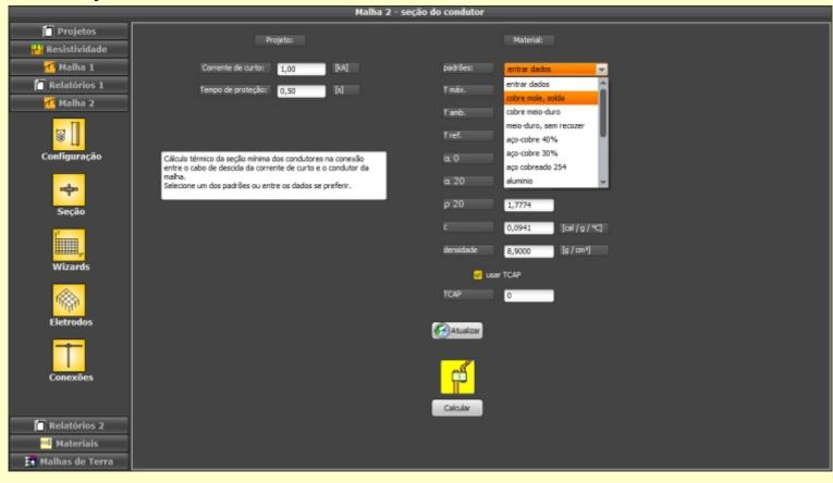
TecAt also has calculations for the conductor section and tolerable potentials (voltages); for conductor section. there are all the standard predefined materials or you can enter your own parameters; for tolerable touch and step potentials, TecAt uses the IEEE-80 formulation (you'll need the grid current and the short-circuit duration)
