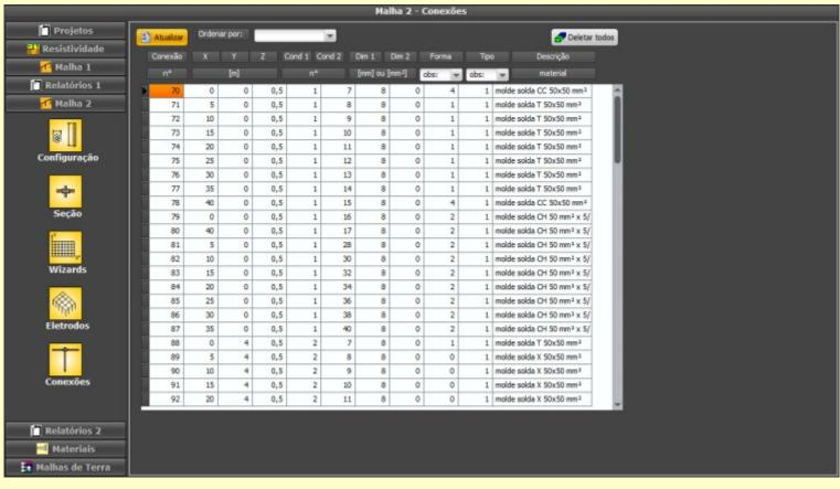
TecAt automatically locates every electrodes junctions of the grid and, using the selected components from the material database, builds the full list of connections
