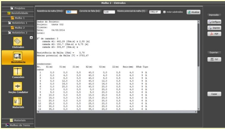
Text report with the resistance calculated and all the electrodes - you can also list the electrodes as divided for the calculations (for better precision)
