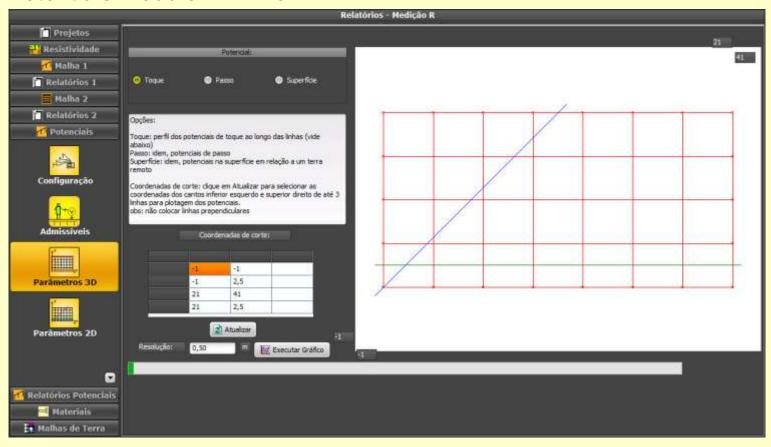
For the 2-D view of touch, step and surface potentials, you can set up to 3 lines at a time, including coordinates outside the grid; as in the 3-D view, you can also set the chart resolution
