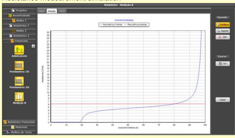
An additional feature of TecAt is the possibility to simulate the resistance measurement after the grid is built on the given soil; that's very handy when you don't have enough space to perform a full measurement
