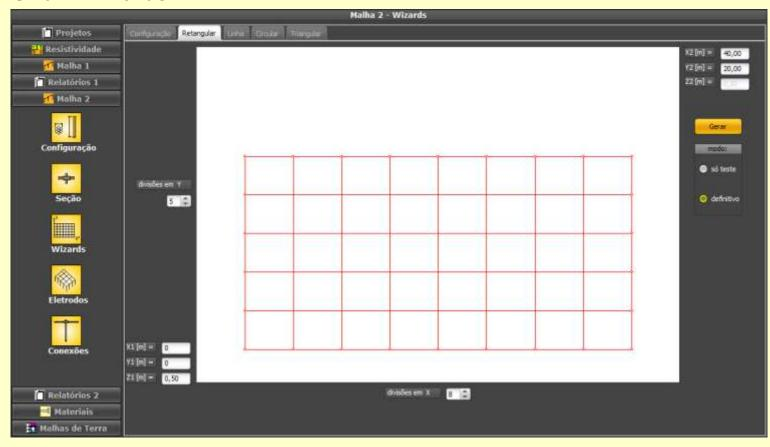
With TecAt 'wizards' you can generate automatically each regular portion of the grid; there are wizards for rectangular, linear, circular (poligon) and triangular portions, and the rectangular can have linear or geometric distance between cable lines (and its rods).
