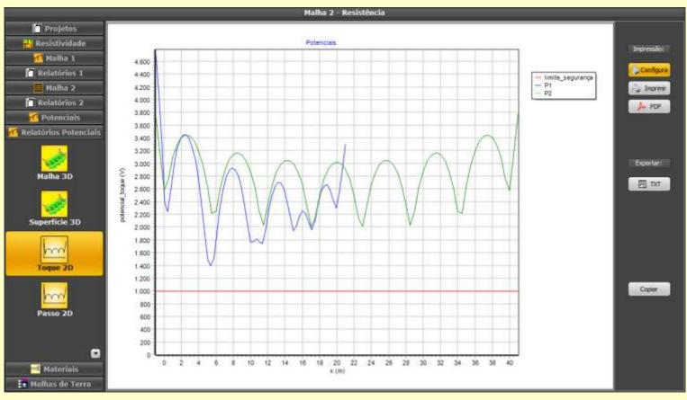
At the 2-D view of touch, step and surface potentials, the potentials along each defined line is plotted, along with the tolerable touch/step potential (calculated separately - see next); for the surface potentials, the red line represents the GPR
