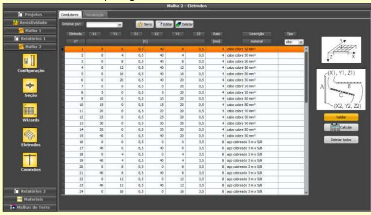
Grid 2 module for complex grids, substations: you can enter each electrode or use the 'wizards' for automatic generation;
