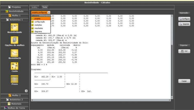
Select the data you want at the report, including deviations for each point and RMS of the whole set, proportioning full certainty of the adjustment between field data and calculated curve.
