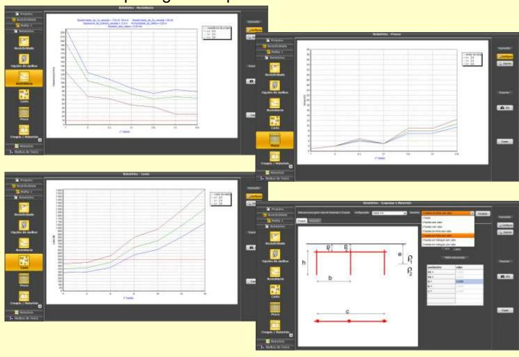
On the Grid 1 module, TecAt calculates instantly 21 different grids with the same configuration but different sizes, presenting comparative charts of resistance, cost and time to build; after you select the best solution for your case, you can generate its descriptive (with draft) and materials reports
