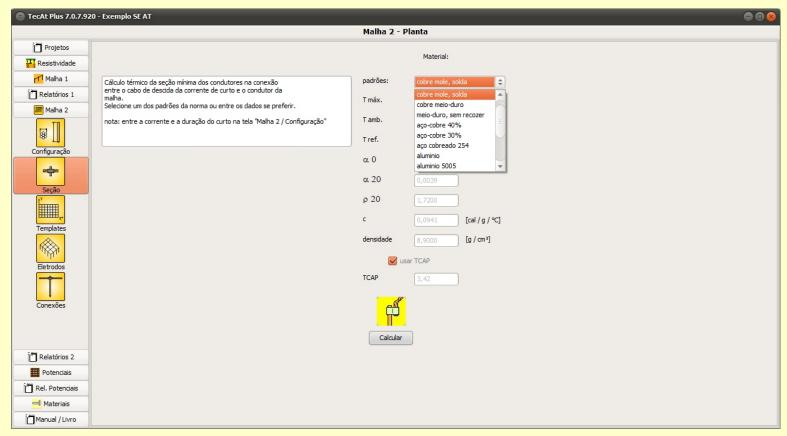
TecAt also calculates the conductor section and the admissible potentials; for the conductor section, all materials from the standard are registered, or you can enter your own values; for the admissible touch and step potentials, TecAt uses the formulations of
